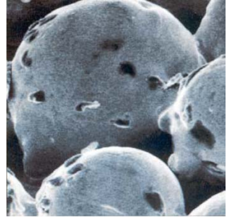
SINTERIP: septum of 5 micron sintered powders under the electron microscope (200x)
